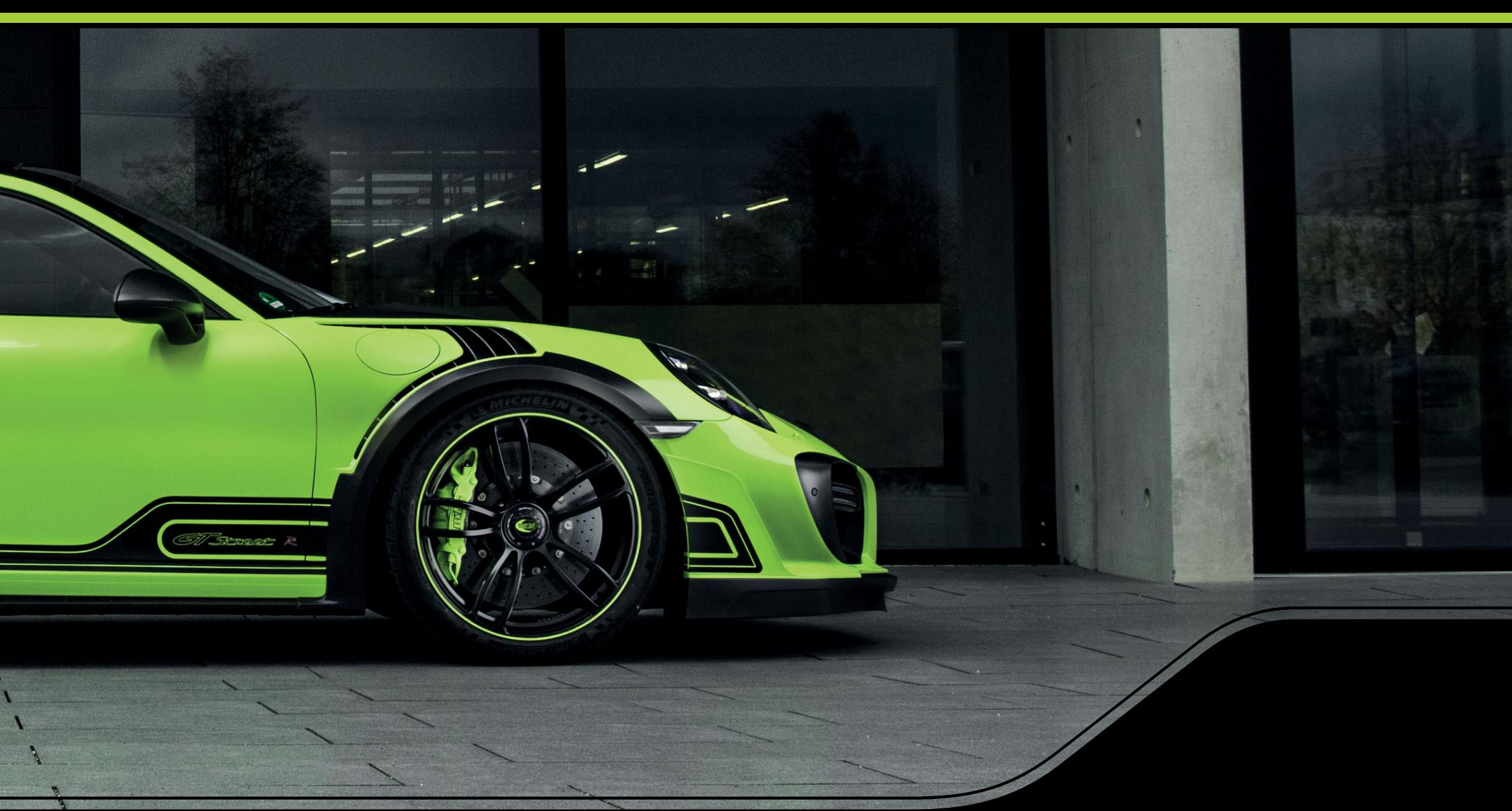
The carbon front fenders feature front wheel arch air outlets. Both, the heat generated by the brakes as well as the overpressure produced by the turning wheels are discharged through racy visible carbon slats. The carbon side skirts continue the GTstreet R design line and interlink the extended wheel arches at front and rear aesthetically. For maximum airflow to the intercoolers, the rear side sections of the GTstreet R feature powerful carbon air intakes.
